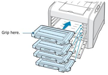
When the toner cartridges are correctly installed, the yellow and black cartridges are not fully inserted. These will be pushed into place when you close the left cover. **15** Close the left cover. Make sure that it is securely latched.
